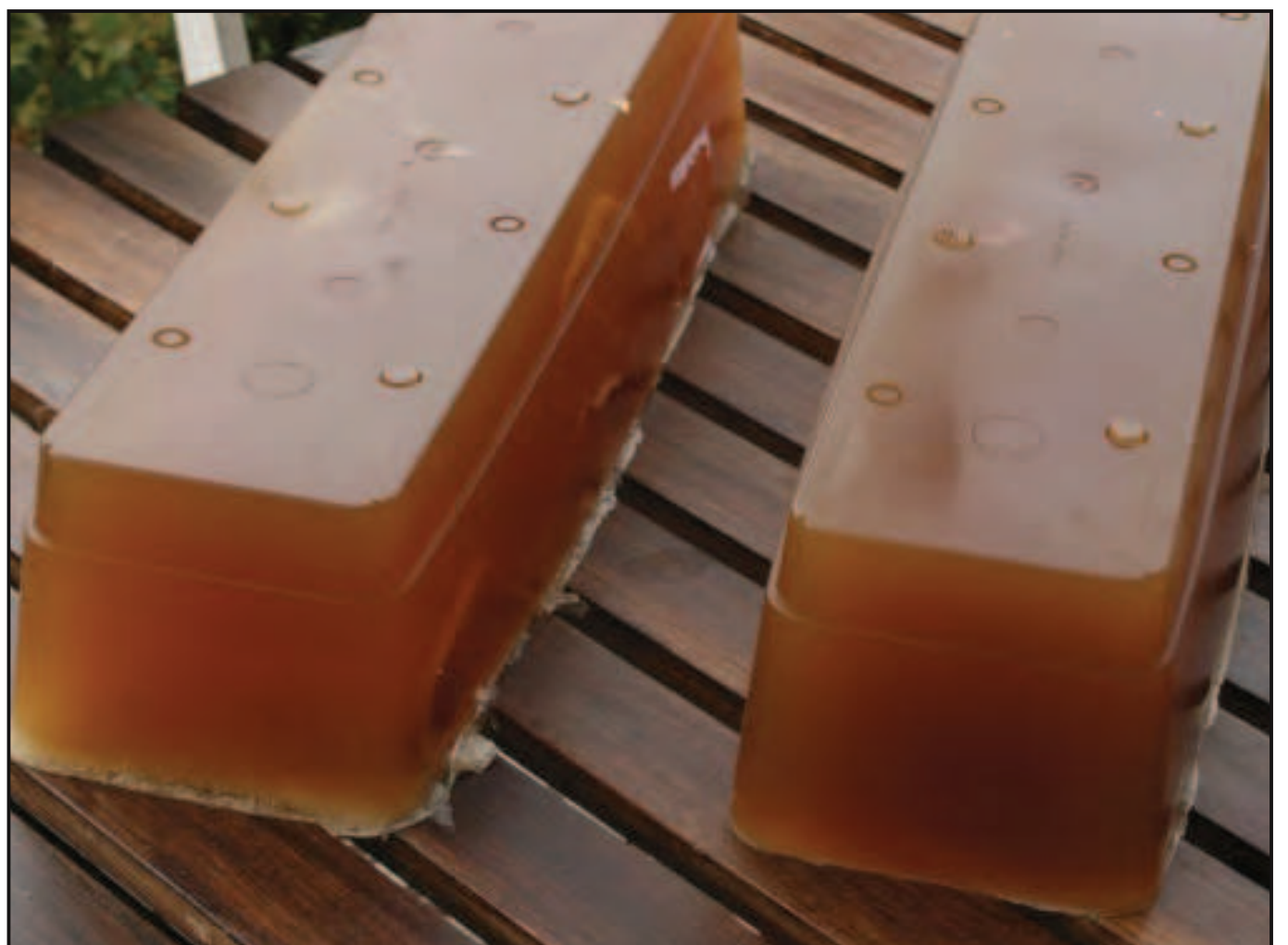
Two 60 x15 x 15 cm gelatin blocks prepared for test shooting
